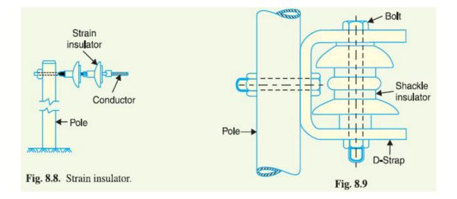
**4. Shackle insulators.** In early days, the shackle insulators were used as strain insulators. But now a days, they are frequently used for low voltage distribution lines. Such insulators can be used either in a horizontal position or in a vertical position. They can be directly fixed to the pole with a bolt or to the cross arm. Fig. shows a shackle insulator fixed to the pole. The conductor in the groove is fixed with a soft binding wire.
