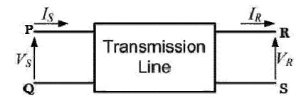
The receiving end is open circuited meaning receiving end current IR = 0. Applying this condition to equation (1) we get.
