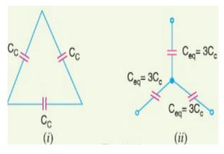
The system of capacitances shown in Fig.(iii) reduces to the equivalent circuit shown in Fig. (i). Therefore, the whole cable is equivalent to three star-connected capacitors each of capacitance
