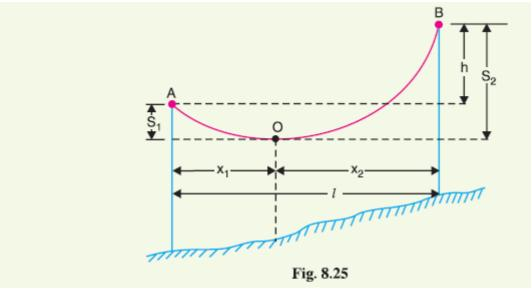
If w is the weight per unit length of the conductor, then,
