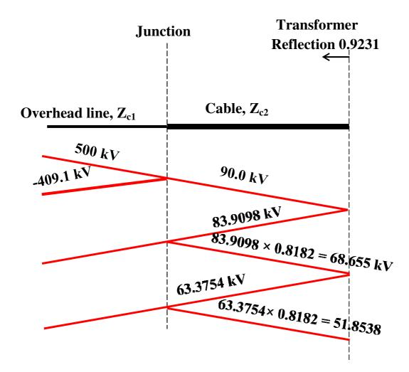
90.9 kV up to 13.2  $\mu sec$  , 243.46 kV from 13.2 to 26.4  $\mu sec$  , rising to 358.69 kV at 26.4  $\mu sec$  .
