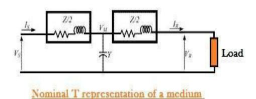
Here also Vs and Vr is the supply and receiving end voltages respectively, and
