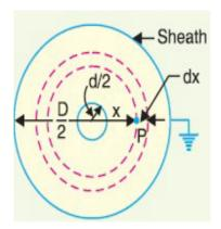
:. Electric flux density at any point P on the considered cylinder is
