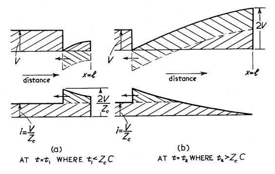
Voltages and currents at a capacitor line termination.
