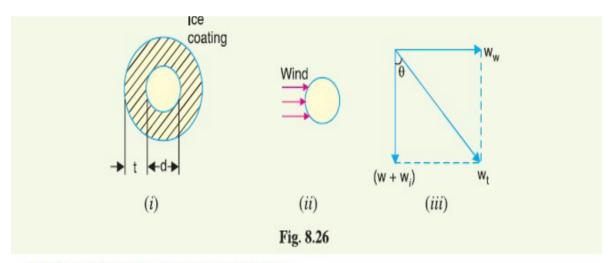
Total weight of conductor per unit length is
