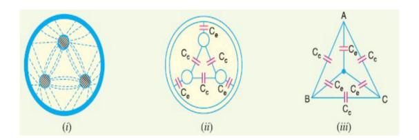
They lay of a belted cable makes it reasonable to assume equality of each Cc and each Ce. The three delta connected capacitances Cc [See Fig.( i)] can be converted into equivalent star connected capacitances as shown in Fig.(ii). It can be easily \*shown that equivalent star capacitance Ceq is equal to three times the delta capacitance Cc i.e. Ceq = 3Cc.
