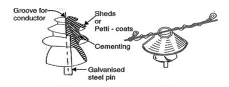
Fig. Pin-type insulator
