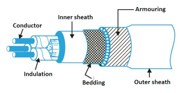
Construction of a cable
