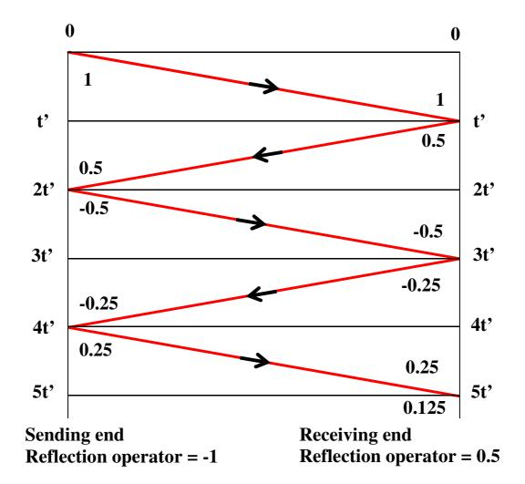
Figure 5: Lattice diagram for line terminated in a resistance
