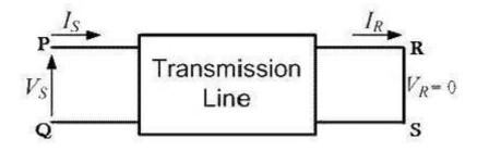
Receiving end is short circuited meaning receiving end voltage VR = 0Applying this condition to equation (1) we get
