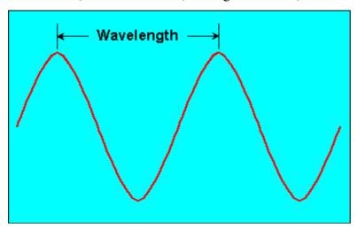
Wavelength is inversely related to  $\underline{\text{frequency}}$ . The higher the frequency of the signal, the shorter the wavelength. If f is the frequency of the signal as measured in megahertz, and w is the wavelength as measured in meters, then
